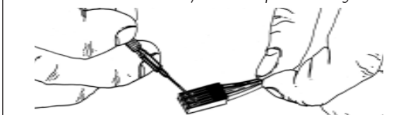
FIGURE 3 With a small standard screwdriver, gently lift plastic prong until wire and metal socket easily slide out of plastic housing.
