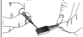
FIGURE 3 With a small std screwdriver, gently lift plastic prong until wire and metal socket easily slide out of plastic housing.
